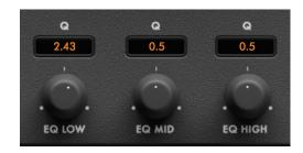
Zone has a 3-band parametric EQ with independent Q controls for each band. The EQ section can be configured to appear after or before the FX section in the signal chain.
