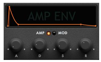
The ATTACK (A), DECAY (D), SUSTAIN (S) and RELEASE (R) portions of the envelopes can be adjusted (in ms) by clicking and dragging the respective knobs. Please note that for shorter ATTACK and DECAY settings, audible clicks may occur in the audio. To eliminate these, click the A or D knob and enter a numerical value a fraction higher than that displayed.
