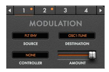
Zone allows up to eight different modulation matrices to be assigned and routed simultaneously.
