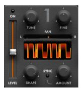
**<u>LEVEL</u>** - Adjusts the relative volume of each oscillator. Clicking the LED at the top switches the oscillator on or off.
