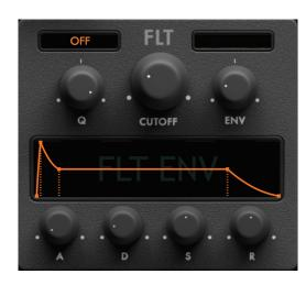
The filter type can be cycled by click and dragging on or clicking in the box to the top left of the CUTOFF control.
