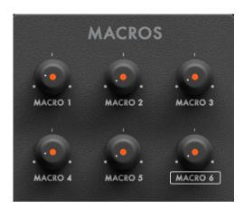
Zone allows up to ten individual controls to be assigned to each of its Macros to be controlled by one knob.
